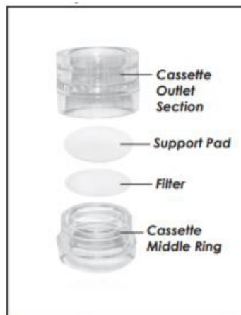
Figure 1. Assemble filter cassette for installation on cyclone
